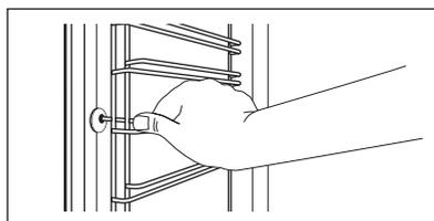
2. Pull the rear end of the shelf support away from the side wall and remove it.
