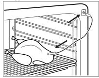
Make sure that the core temperature sensor stays in the meat and in the socket during the cooking. When you use the core temperature sensor for the first time, the default core temperature is 60 °C. While flashes, you can use the knob for the temperature to change the default core temperature.
