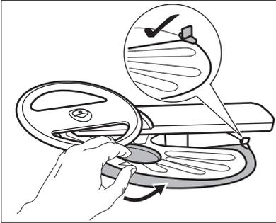
7. Reassemble the filters (B) and (C).
