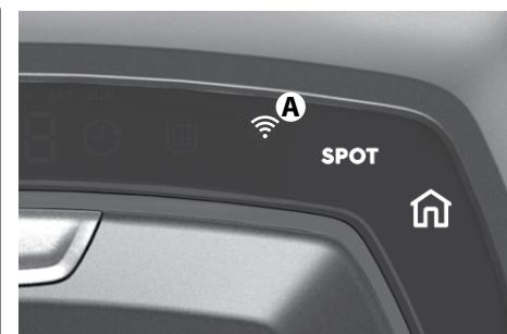
**3. When the setup is completed,** turn the robot back to its normal position. The WiFi symbol (A) will be lit up to indicate that the robot is connected to your home network. **Note:** it could take a few moments for the robot clock to automatically synchronise with your mobile device. **Note:** Pulsing WiFi symbol indicates that the robot is trying to connect to the network.
