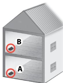
**Cleaning of a house with more than one floor can be facilitated by using an extra charging base on each floor. (ANC: 406000071)**
