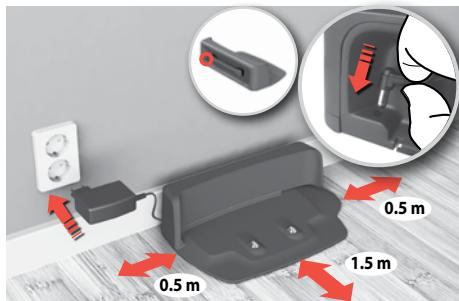
**1. Place the Charging base** on the floor against the wall.
