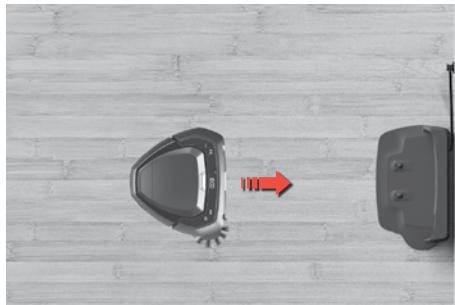
**When cleaning is completed**, the robot automatically returns to the charging base.
