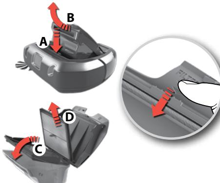
**Rengjøring av filteret****Czyszczenie filtra**
