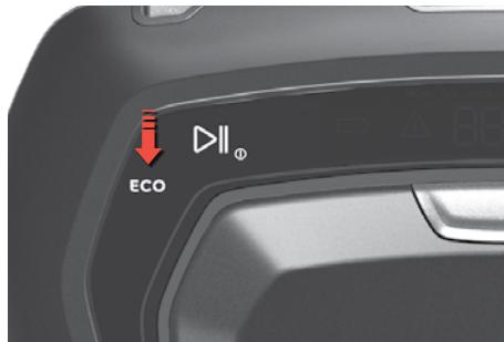
**ECO mode:** For a lighter cleaning, press the ECO button to reduce the power, prolong the running time and reduce noise level. The robot will stay in ECO mode until the button is pressed again.
