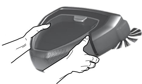
**Always carry the robot with two hands keeping the front up. Manual moving of the robot:**
