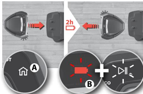
**Should recharging be needed during cleaning,** the home button will light up and the robot will return to the charging base. Home button (A) is lit. The battery and Play/Pause button (B) flash to indicate that the robot is charging and that it will resume where it stopped.
