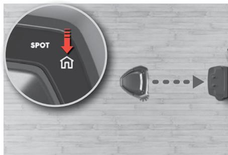
**Stop cleaning and send the robot to the charging base:** Press the Home button. If the robot is not started from the charging base, it will return to the starting position.
