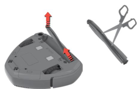
**2. Pull out the Brush roll and clean the brush and bearings.** Remove entangled threads by snipping them away with scissors. Refit in reverse order.
