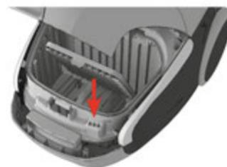
8. **Replace the motor filter when dirty or after every 5th s-bag®**: Push the filter holder down and pull it out. Exchange the filter and close the lid.
