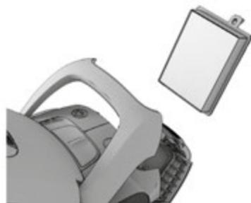
**4. Lift out the filter and check the color of the frame:**
