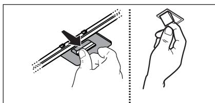
**4.2 NON-washable activated charcoal filter** - The saturation of the **charcoal filter** occurs after more or less prolonged use, depending on the type of cooking and the regularity of cleaning of the grease filter. In any case it is necessary to replace the cartridge at least every four months. The charcoal filter may NOT be washed or regenerated.
