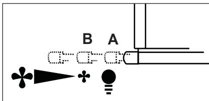
Use the high suction speed in cases of concentrated kitchen vapours. It is recommended that the cooker hood suction is switched on for 5 minutes prior to cooking and to leave in operation during cooking and for another 15 minutes approximately after terminating cooking.
