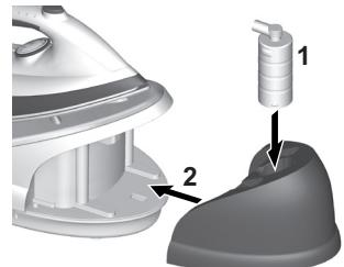
**6. Insert the water tank** into the base unit. Ensure that the water tank latches securely into place.
