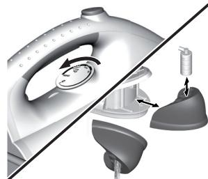
6. Turn the **temperature dial** back to its minimum setting. Then, turn off the steam generator iron and disconnect it from the mains supply. **Empty the water tank** and allow the iron to cool completely prior to storage.
